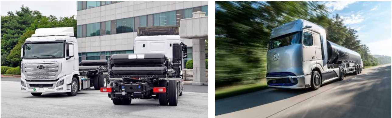
Fig. 5.21: left: XCIENT fuel cell truck (Hyundai); right: GenH 2 with LH 2 tanks of Daimler Trucks (Daimler Trucks)
