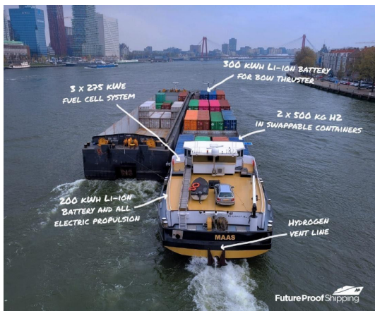
Fig. 5.17 : Hydrogen fuel cell hybrid electric container ship by Holland Shipyards Group (cf. VPO)
